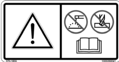
Fig. 40: Do not drill holes or weld the ROPS structure
