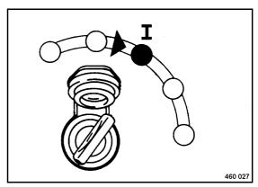
Turn the ignition key (Fig. 57) to position "I".
