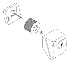
**Note:** If the motor starts smoking and if the motor output drops at the same time, this indicates that the filter is clogged.
