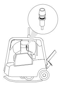
▶ Rev the engine briefly to its maximum speed. If the rubber bellows contract and cover the green field "2" in the process, the air cleaner system must be serviced. If you are working in dusty conditions, check the rubber bellows several times a day.
