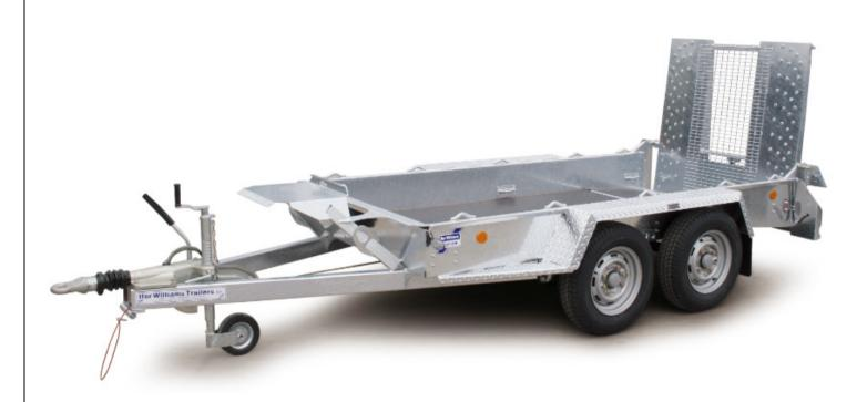
Note: Axles, tyres and suspension are rated at 1800kg per axle
